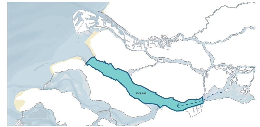
Figure 6.17 Increased water storage capacity of the Haringvliet. Subsystem: Soil & Water
